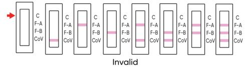
**Check** to see if a pink to red line is visible at the control line 'C' in the results window. If a line is not visible at "C", even if any other line is visible in the results window, the result is considered invalid.
