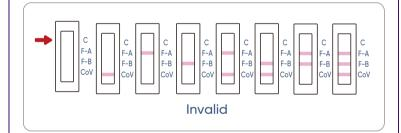
Check to see if a pink to red line is visible at the control line 'C' in the results window. If a line is not visible at 'C', even if any other line is visible in the results window, the result is considered invalid.
